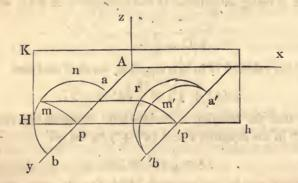
K L parallel to the plane (x, z), the section of the surface by this plane will be a straight line; since, for all the points of this section, y being equal to A p, if we represent A p by a constant c, the quantities  $\varphi y, \psi y$ will become  $\varphi c, \psi c$ , and, consequently, may be replaced by two constants, a, b, so that the equation
